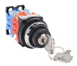
Fuji Electric selector switch, 30mm, 3-position, spring return from left and right to center, key removable center position, (2) N.O./ (2) N.C. contact(s), plastic base, metal bezel, Operator: black, key, 35mm, round, plastic.
