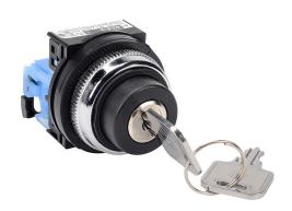
Fuji Electric selector switch, 30mm, 2-position, spring return from right, key removable left position, (1) N.O. contact(s), plastic base, metal bezel, Operator: black, key, 35mm, round, plastic.
