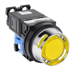
Fuji Electric pushbutton, 30mm, momentary, LED illuminated, (1) N.O. contact(s), plastic base, metal bezel, guarded, Operator: yellow, extended, 35mm, round, plastic, 115-127 VAC, transformer.
