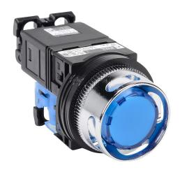
Fuji Electric pushbutton, 30mm, momentary, LED illuminated, (1) N.O. contact(s), plastic base, metal bezel, guarded, Operator: blue, extended, 35mm, round, plastic, 115-127 VAC, transformer.
