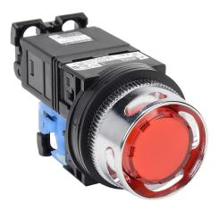
Fuji Electric pushbutton, 30mm, momentary, LED illuminated, (1) N.O. contact(s), plastic base, metal bezel, guarded, Operator: red, extended, 35mm, round, plastic, 115-127 VAC, transformer.
