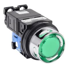
Fuji Electric pushbutton, 30mm, momentary, LED illuminated, (1) N.O. contact(s), plastic base, metal bezel, guarded, Operator: green, extended, 35mm, round, plastic, 115-127 VAC, transformer.
