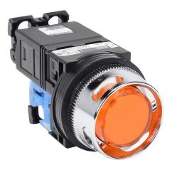
Fuji Electric pushbutton, 30mm, momentary, LED illuminated, (1) N.O. contact(s), plastic base, metal bezel, guarded, Operator: orange, extended, 35mm, round, plastic, 115-127 VAC, transformer.
