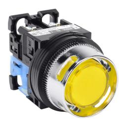
Fuji Electric pushbutton, 30mm, momentary, LED illuminated, (1) N.O. contact(s), plastic base, metal bezel, guarded, Operator: yellow, extended, 35mm, round, plastic, 24 VAC/VDC, full voltage.
