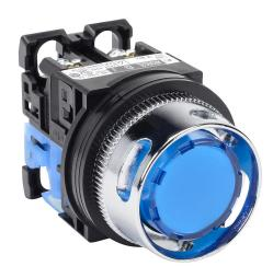
Fuji Electric pushbutton, 30mm, momentary, LED illuminated, (1) N.O. contact(s), plastic base, metal bezel, guarded, Operator: blue, extended, 35mm, round, plastic, 24 VAC/VDC, full voltage.
