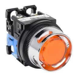
Fuji Electric pushbutton, 30mm, momentary, LED illuminated, (1) N.O. contact(s), plastic base, metal bezel, guarded, Operator: orange, extended, 35mm, round, plastic, 24 VAC/VDC, full voltage.
