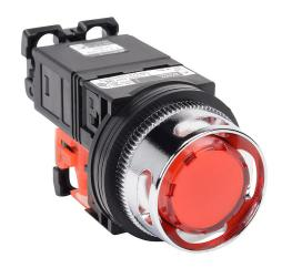
Fuji Electric pushbutton, 30mm, momentary, LED illuminated, (1) N.C. contact(s), plastic base, metal bezel, guarded, Operator: red, extended, 35mm, round, plastic, 115-127 VAC, transformer.
