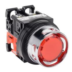
Fuji Electric pushbutton, 30mm, momentary, LED illuminated, (1) N.C. contact(s), plastic base, metal bezel, guarded, Operator: red, extended, 35mm, round, plastic, 24 VAC/VDC, full voltage.
