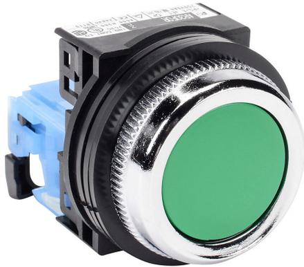
Fuji Electric pushbutton, 30mm, momentary, (1) N.O. contact(s), plastic base, metal bezel, Operator: green, flush, 35mm, round, plastic.
