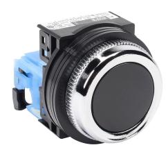
Fuji Electric pushbutton, 30mm, momentary, (1) N.O. contact(s), plastic base, metal bezel, Operator: black, flush, 35mm, round, plastic.
