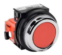
Fuji Electric pushbutton, 30mm, momentary, (1) N.C. contact(s), plastic base, metal bezel, Operator: red, flush, 35mm, round, plastic.
