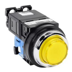
Fuji Electric pushbutton, 30mm, momentary, LED illuminated, (1) N.O. contact(s), plastic base, metal bezel, Operator: yellow, extended, 35mm, round, plastic, 115-127 VAC, transformer.
