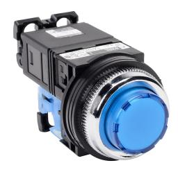
Fuji Electric pushbutton, 30mm, momentary, LED illuminated, (1) N.O. contact(s), plastic base, metal bezel, Operator: blue, extended, 35mm, round, plastic, 115-127 VAC, transformer.
