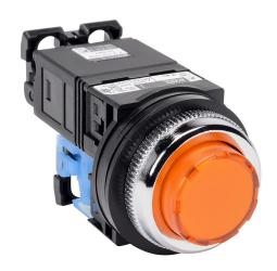
Fuji Electric pushbutton, 30mm, momentary, LED illuminated, (1) N.O. contact(s), plastic base, metal bezel, Operator: orange, extended, 35mm, round, plastic, 115-127 VAC, transformer.
