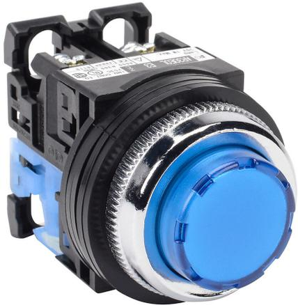
Fuji Electric pushbutton, 30mm, momentary, LED illuminated, (1) N.O. contact(s), plastic base, metal bezel, Operator: blue, extended, 35mm, round, plastic, 24 VAC/VDC, full voltage.
