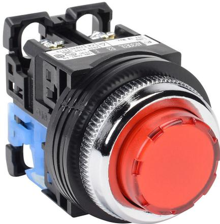
Fuji Electric pushbutton, 30mm, momentary, LED illuminated, (1) N.O. contact(s), plastic base, metal bezel, Operator: red, extended, 35mm, round, plastic, 24 VAC/VDC, full voltage.
