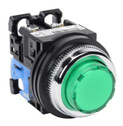
Fuji Electric pushbutton, 30mm, momentary, LED illuminated, (1) N.O. contact(s), plastic base, metal bezel, Operator: green, extended, 35mm, round, plastic, 24 VAC/VDC, full voltage.
