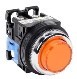
Fuji Electric pushbutton, 30mm, momentary, LED illuminated, (1) N.O. contact(s), plastic base, metal bezel, Operator: orange, extended, 35mm, round, plastic, 24 VAC/VDC, full voltage.
