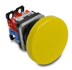
Fuji Electric pushbutton, 30mm, momentary, (1) N.O./(1) N.C. contact(s), metal base, metal bezel, Operator: yellow, mushroom, 65mm, round, plastic.
