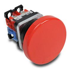
Fuji Electric pushbutton, 30mm, momentary, (1) N.O./(1) N.C. contact(s), metal base, metal bezel, Operator: red, mushroom, 65mm, round, plastic.
