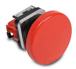
Fuji Electric pushbutton, 30mm, momentary, (1) N.C. contact(s), metal base, metal bezel, Operator: red, mushroom, 65mm, round, plastic.
