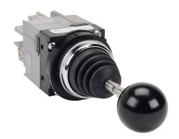
Fuji Electric selector switch, IP65, 30mm, 4-position, momentary, (4) N.O. contact(s), plastic base, metal bezel, Operator: black, joystick, 41mm, round, plastic.
