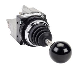
Fuji Electric selector switch, IP65, 30mm, 2-position, maintained, (2) N.O. contact(s), plastic base, metal bezel, Operator: black, joystick, 41mm, round, plastic.
