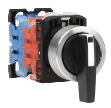
Fuji Electric selector switch, 22mm, 3-position, spring return to center from right or left, (2) N.O./(2) N.C. contact(s), plastic base, metal bezel, Operator: black, lever, 30mm, round, plastic.
