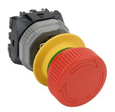
Fuji Electric emergency stop pushbutton, IP65, 22mm, push to lock, pull or turn to reset, (1) N.O./(2) N.C. contact(s), plastic base, plastic bezel, yellow, Operator: red, mushroom, 40mm, mushroom, plastic.
