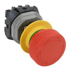
Fuji Electric emergency stop pushbutton, IP65, 22mm, push to lock, pull or turn to reset, (1) N.O./(2) N.C. contact(s), plastic base, plastic bezel, yellow, Operator: red, mushroom, 40mm, mushroom, plastic.
