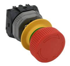
Fuji Electric emergency stop pushbutton, IP65, 22mm, push to lock, pull or turn to reset, (1) N.C. contact(s), plastic base, plastic bezel, yellow, Operator: red, mushroom, 40mm, mushroom, plastic.
