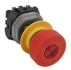
Fuji Electric emergency stop pushbutton, IP65, 22mm, push to lock, pull or turn to reset, interlocked LED illuminated, (1) N.O./(2) N.C. contact(s), plastic base, plastic bezel, yellow, Operator: red, mushroom, 40mm, mushroom, plastic, 24 VAC/VDC, full voltage.
