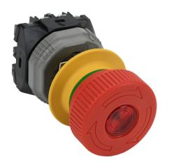
Fuji Electric emergency stop pushbutton, IP65, 22mm, push to lock, pull or turn to reset, interlocked LED illuminated, (1) N.O./(2) N.C. contact(s), plastic base, plastic bezel, yellow, Operator: red, mushroom, 40mm, mushroom, plastic, 24 VAC/VDC, full voltage.
