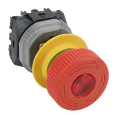
Fuji Electric emergency stop pushbutton, IP65, 22mm, push to lock, pull or turn to reset, LED illuminated, (1) N.C. contact(s), plastic base, plastic bezel, yellow, Operator: red, mushroom, 40mm, mushroom, plastic, 24 VAC/VDC, full voltage.
