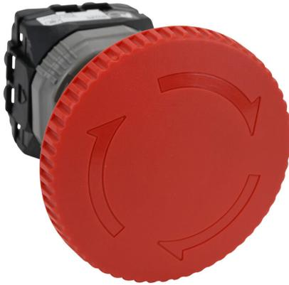
Fuji Electric emergency stop pushbutton, IP65, 22mm, push to lock, pull or turn to reset, (1) N.O./(2) N.C. contact(s), plastic base, plastic bezel, yellow, Operator: red, mushroom, 65mm, mushroom, plastic.
