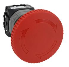
Fuji Electric emergency stop pushbutton, IP65, 22mm, push to lock, pull or turn to reset, (1) N.O./(2) N.C. contact(s), plastic base, plastic bezel, yellow, Operator: red, mushroom, 65mm, mushroom, plastic.
