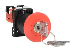
Fuji Electric emergency stop pushbutton, 22mm, key operated release, (1) N.C. contact(s), plastic base, plastic bezel, Operator: red, mushroom, 40mm, round, plastic.
