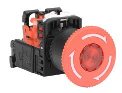
Fuji Electric pushbutton, 22mm, twist-to-release, LED illuminated, (1) N.C. contact(s), plastic base, plastic bezel, Operator: red, mushroom, 40mm, round, plastic, 115-127 VAC, transformer.
