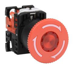
Fuji Electric pushbutton, 22mm, twist-to-release, LED illuminated, (1) N.C. contact(s), plastic base, plastic bezel, Operator: red, mushroom, 40mm, round, plastic, 24 VAC/VDC, full voltage.
