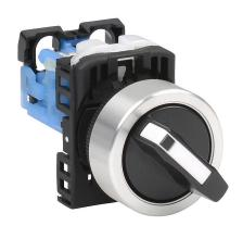
Fuji Electric selector switch, 22mm, 2-position, maintained, (1) N.O. contact(s), plastic base, metal bezel, Operator: black, knob, 30mm, round, plastic.
