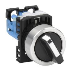
Fuji Electric selector switch, 22mm, 2-position, spring return from right, (1) N.O. contact(s), plastic base, metal bezel, Operator: black, knob, 30mm, round, plastic.
