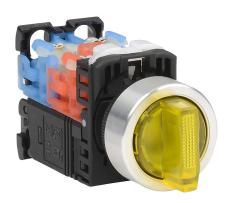
Fuji Electric selector switch, 22mm, 3-position, spring return to center from left, maintained right, LED illuminated, (1) N.O./(1) N.C. contact(s), plastic base, metal bezel, Operator: yellow, knob, 30mm, round, plastic, 115-127 VAC, transformer.
