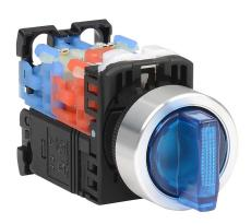
Fuji Electric selector switch, 22mm, 3-position, spring return to center from left, maintained right, LED illuminated, (1) N.O./(1) N.C. contact(s), plastic base, metal bezel, Operator: blue, knob, 30mm, round, plastic, 115-127 VAC, transformer.
