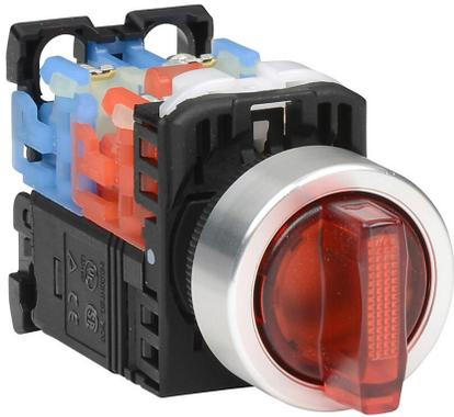
Fuji Electric selector switch, 22mm, 3-position, spring return to center from left, maintained right, LED illuminated, (1) N.O./ (1) N.C. contact(s), plastic base, metal bezel, Operator: red, knob, 30mm, round, plastic, 115-127 VAC, transformer.
