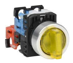
Fuji Electric selector switch, 22mm, 3-position, spring return to center from left, maintained right, LED illuminated, (1) N.O./(1) N.C. contact(s), plastic base, metal bezel, Operator: yellow, knob, 30mm, round, plastic, 24 VAC/VDC, full voltage.
