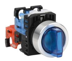
Fuji Electric selector switch, 22mm, 3-position, spring return to center from left, maintained right, LED illuminated, (1) N.O./(1) N.C. contact(s), plastic base, metal bezel, Operator: blue, knob, 30mm, round, plastic, 24 VAC/VDC, full voltage.
