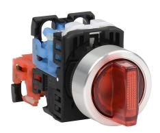
Fuji Electric selector switch, 22mm, 3-position, spring return to center from left, maintained right, LED illuminated, (1) N.O./(1) N.C. contact(s), plastic base, metal bezel, Operator: red, knob, 30mm, round, plastic, 24 VAC/VDC, full voltage.
