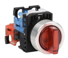
Fuji Electric selector switch, 22mm, 3-position, spring return to center from left, maintained right, LED illuminated, (1) N.O./(1) N.C. contact(s), plastic base, metal bezel, Operator: red, knob, 30mm, round, plastic, 24 VAC/VDC, full voltage.
