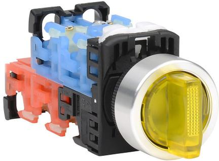
Fuji Electric selector switch, 22mm, 3-position, maintained, LED illuminated, (2) N.O./ (2) N.C. contact(s), plastic base, metal bezel, Operator: yellow, knob, 30mm, round, plastic, 24 VAC/VDC, full voltage.
