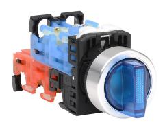
Fuji Electric selector switch, 22mm, 3-position, maintained, LED illuminated, (2) N.O./(2) N.C. contact(s), plastic base, metal bezel, Operator: blue, knob, 30mm, round, plastic, 24 VAC/VDC, full voltage.
