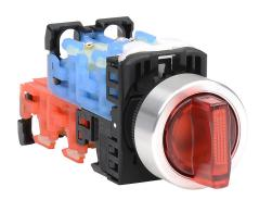
Fuji Electric selector switch, 22mm, 3-position, maintained, LED illuminated, (2) N.O./(2) N.C. contact(s), plastic base, metal bezel, Operator: red, knob, 30mm, round, plastic, 24 VAC/VDC, full voltage.
