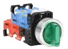
Fuji Electric selector switch, 22mm, 3-position, maintained, LED illuminated, (2) N.O./(2) N.C. contact(s), plastic base, metal bezel, Operator: green, knob, 30mm, round, plastic, 24 VAC/VDC, full voltage.
