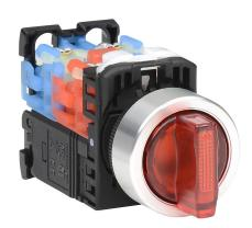
Fuji Electric selector switch, 22mm, 3-position, maintained, LED illuminated, (1) N.O./(1) N.C. contact(s), plastic base, metal bezel, Operator: red, knob, 30mm, round, plastic, 115-127 VAC, transformer.
