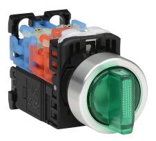
Fuji Electric selector switch, 22mm, 3-position, maintained, LED illuminated, (1) N.O./(1) N.C. contact(s), plastic base, metal bezel, Operator: green, knob, 30mm, round, plastic, 115-127 VAC, transformer.
